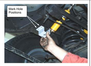
Place swaybar extension bracket No. 3751649 in position as shown.
