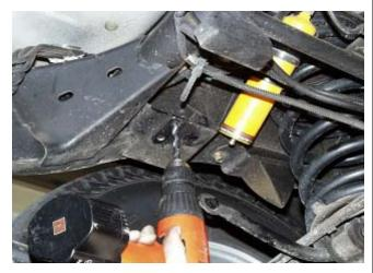
Drill two 8mm holes where previously marked.
