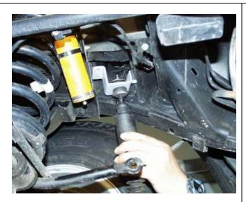
Assemble the swaybar link and extension bracket as shown.
