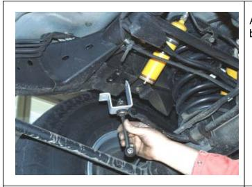
Assemble the swaybar link and extension bracket as shown.
