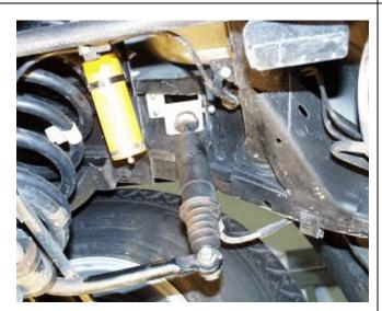
Bolt in position using the existing chassis holes and the bolts supplied.
